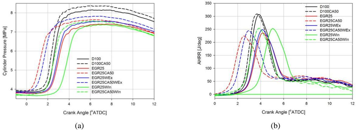
Fig. 7 The variation of cylinder pressure and heat release rate with crank angle for EGR of 25% with water injection of 40 mg/cycle into intake and exhaust manifolds (a)  $p-\theta$  (b) AHRR
