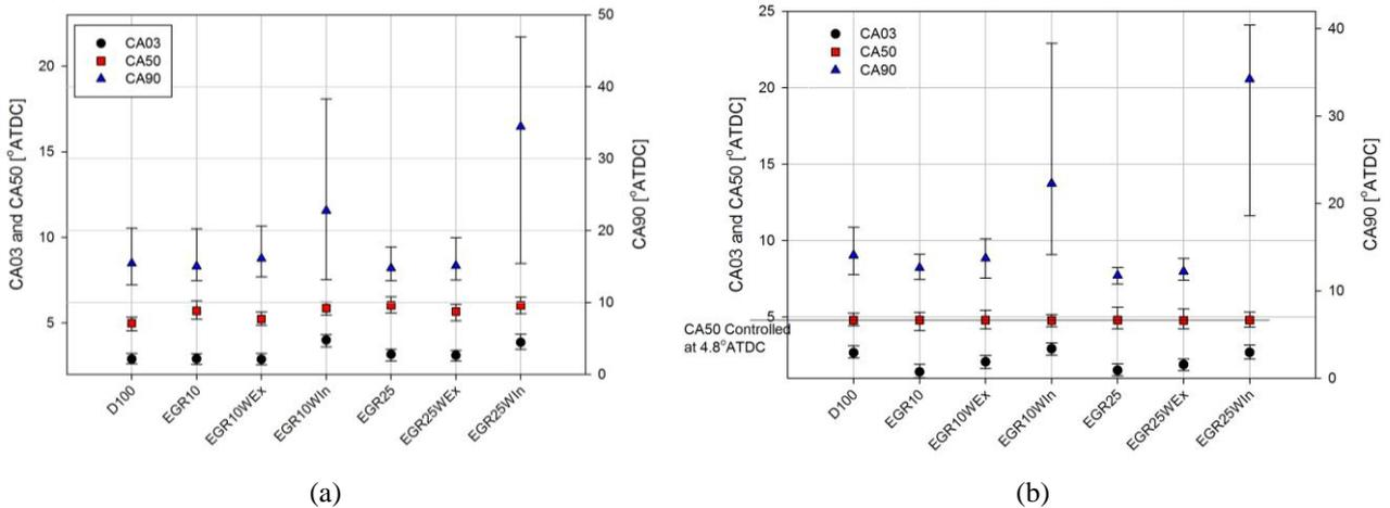
Fig. 8 Ignition delay and combustion phasing for 10% and 25% EGR and water injection into intake and exhaust manifolds (a) Without CA50 control (b) With CA50 control
