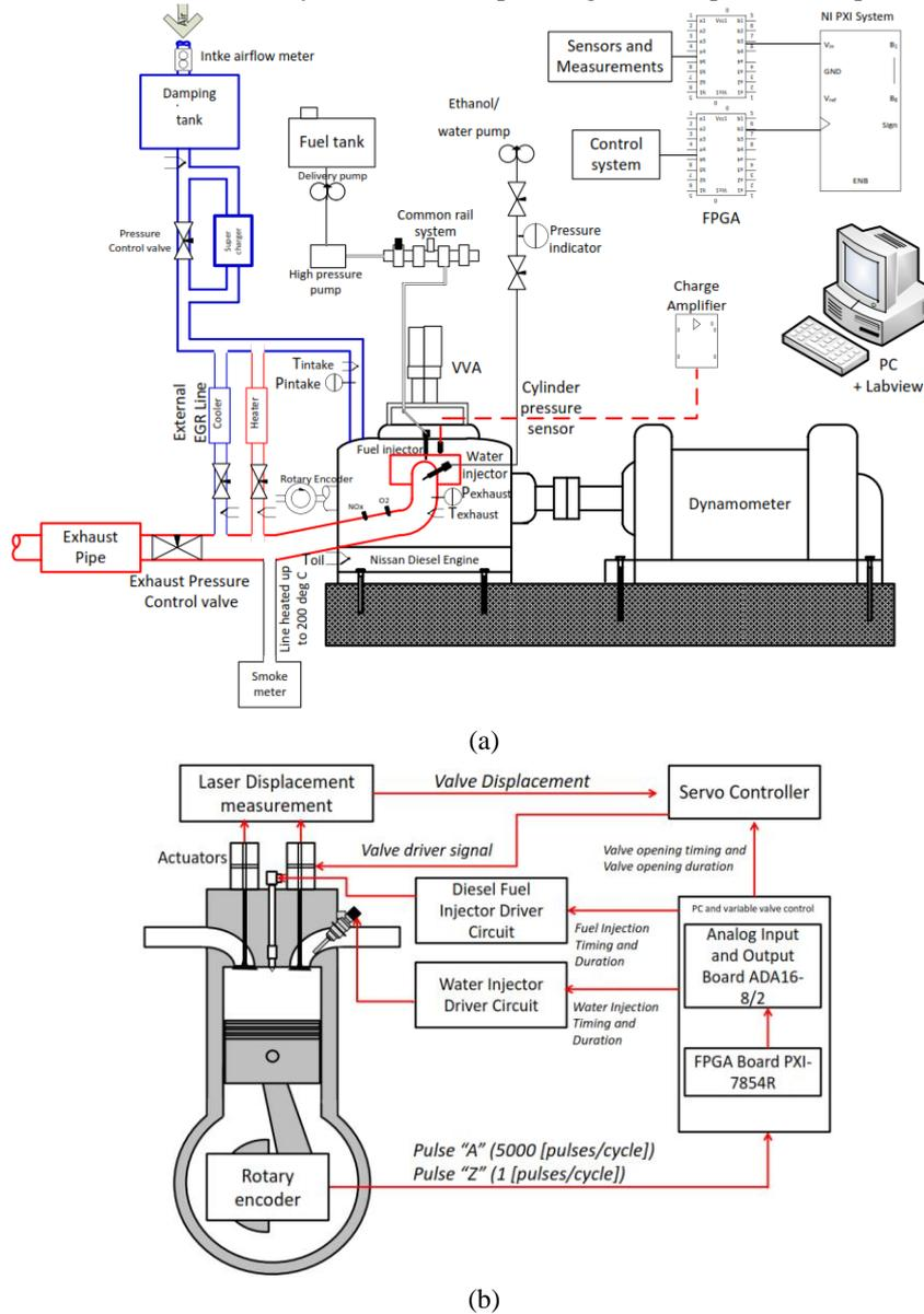
Fig. 1 Diesel engine test system (a) Experimental system overview and measurement instrumentation (b) Variable valve actuating, diesel fuel injection and water injection control system
