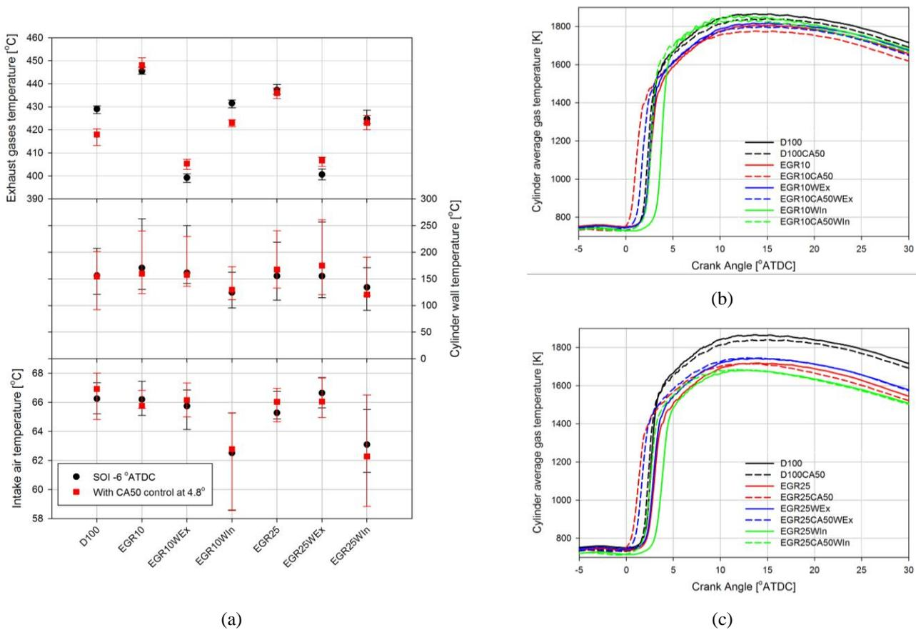
Fig. 9 Temperature measurement for 10% and 25% EGR and water injection into intake and exhaust manifolds (a) Intake air, cylinder wall and exhaust gases temperatures (b) Average gas temperature for 10% EGR (c) Average gas temperature for 25% EGR with and without CA50
