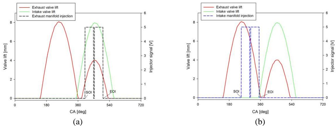
Fig. 4 Water injection timing and duration with valve timing for (a) Exhaust injection (b) Intake injection.
