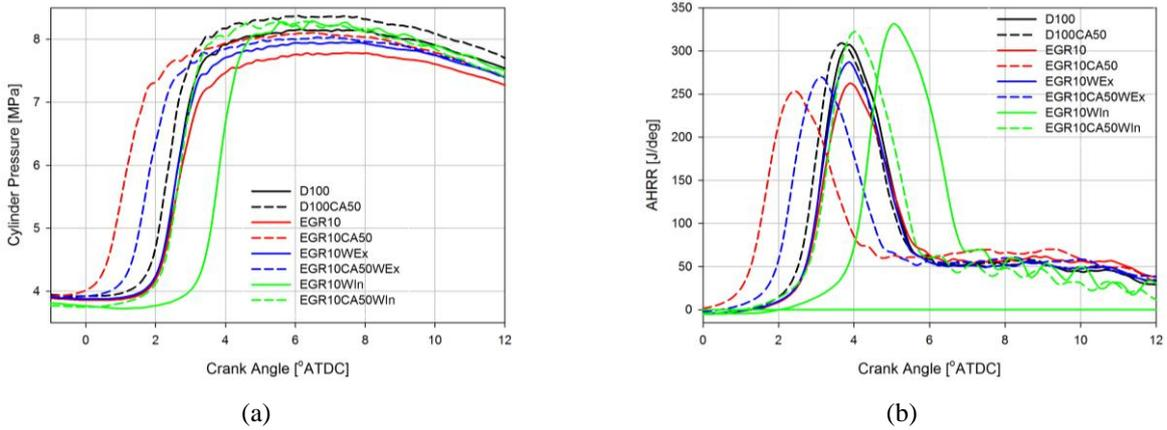
Fig. 6 The variation of cylinder pressure and heat release rate with crank angle for EGR of 10% with water injection of 40 mg/cycle into intake and exhaust manifolds (a)  $p-\theta$  (b) AHRR
