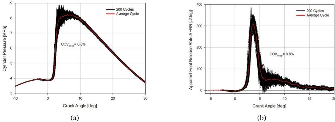
Fig. 2 The average cycle of the conventional diesel combustion that was used to represent the 200 cycles with  $COV_{imep} = 0.8\%$  (a)  $p$ - $\theta$  diagram (b) AHRR.
