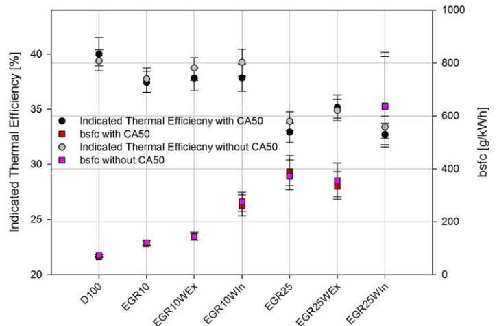
Fig. 11 Indicated thermal efficiency and bsfc for 10% and 25% EGR and water injection into intake and exhaust manifold with and without CA50 control
