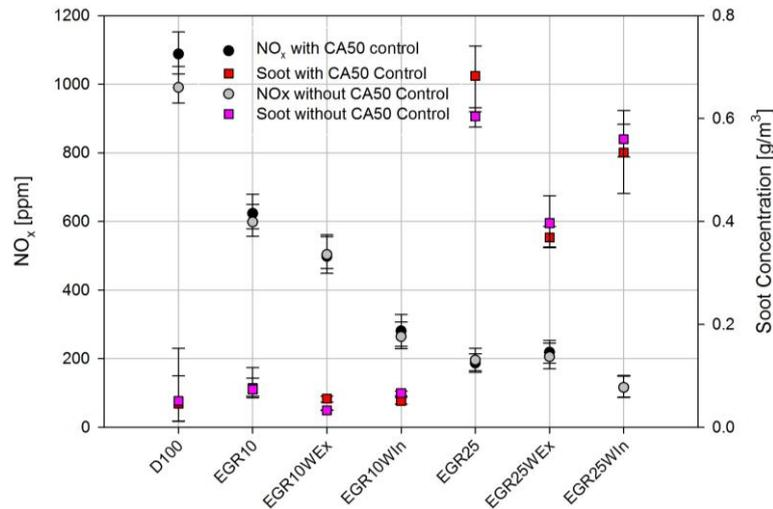
Fig. 12 Soot and NO<sub>x</sub> emissions for 10% and 25% EGR with water injection into intake and exhaust manifold with and without CA50 control
