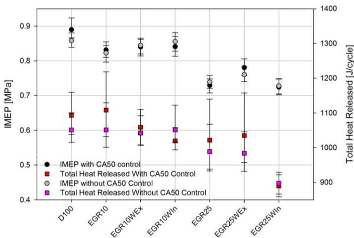
Fig. 10 IMEP and total heat released for 10% and 25% EGR and water injection into intake and exhaust manifold with and without CA50 control
