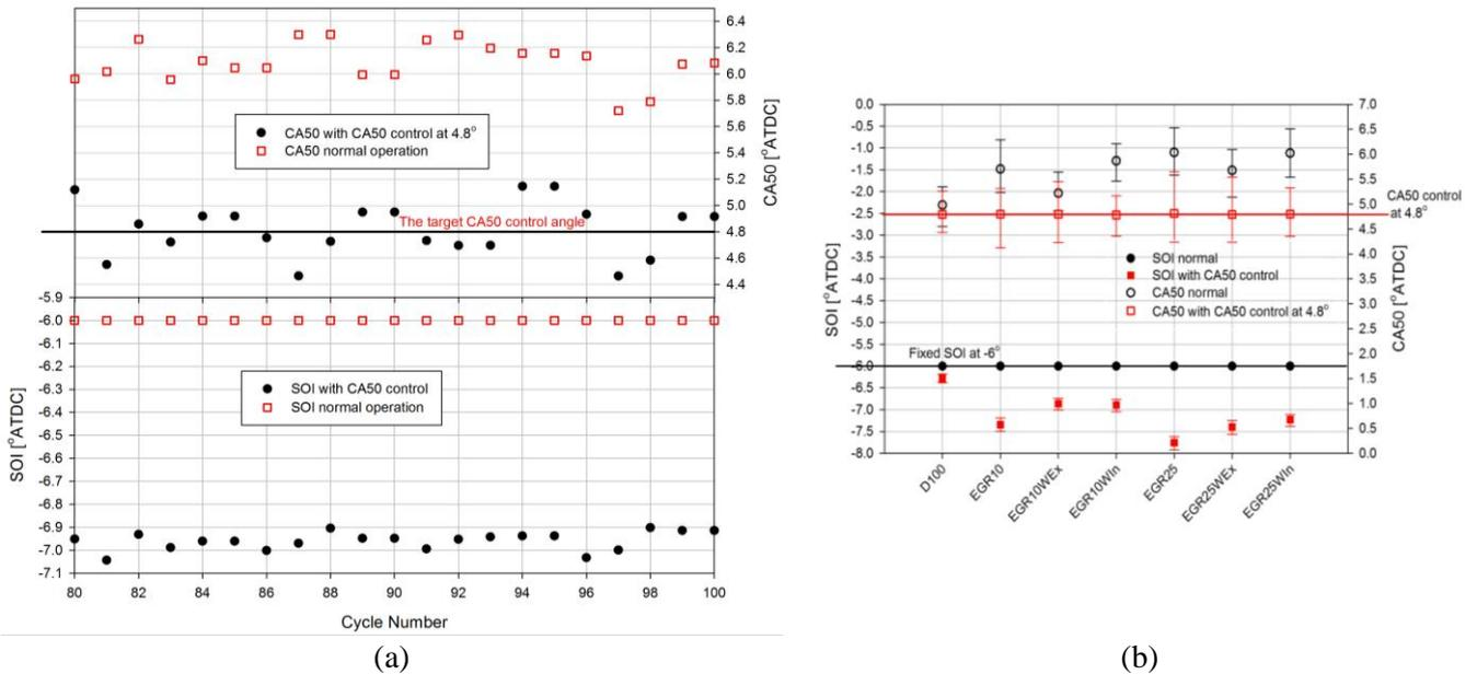
Fig. 5 Definition of CA50 control (a) Conventional diesel cycle-to-cycle variation of SOI for CA50 control at 4.8° for 20 consecutive cycles (b) SOI and CA50 for the different condition with and without CA50 control.
